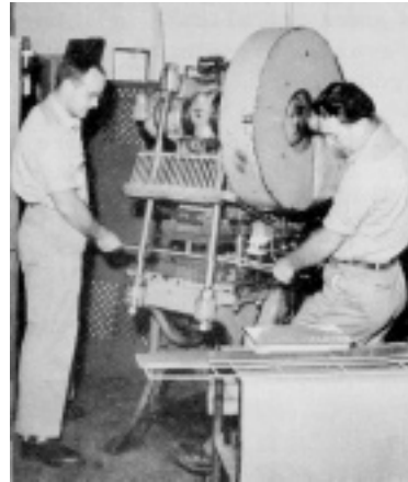
Figure 48.17. Punching core blanks for a picture frame assembly from sheared strips.
