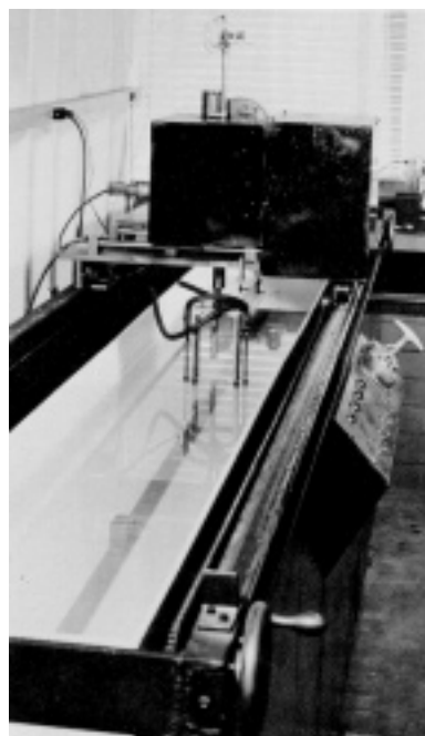
Figure 48.8. Ultrasonic inspection apparatus.
