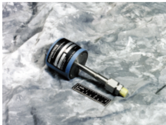
Figure 32.1. Capacitance diaphragm pressure transducer.
