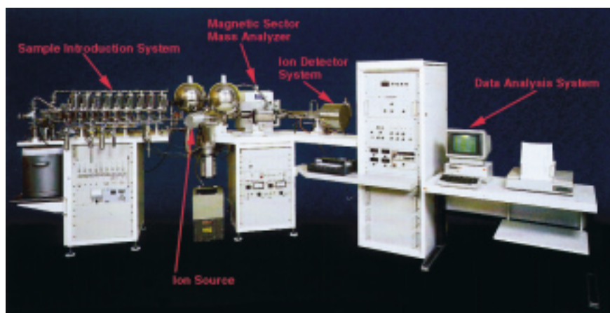
Figure 31.4.1. A magnetic sector mass spectrometer equipped with an electron bombardment ion source. (Courtesy of Finnigan Corporation.)
