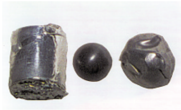
Figure 1.2. From left to right, clad plutonium pellet, highly enriched uranium sphere, and deformed lead sphere.
