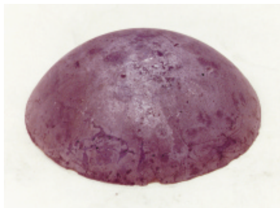
Figure 1.4. Metallic plutonium button produced by direct oxide reduction.
