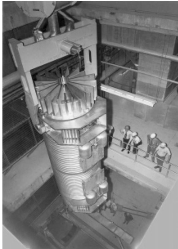
Figure 1.8. Shipping cask for transporting spent nuclear fuel.
