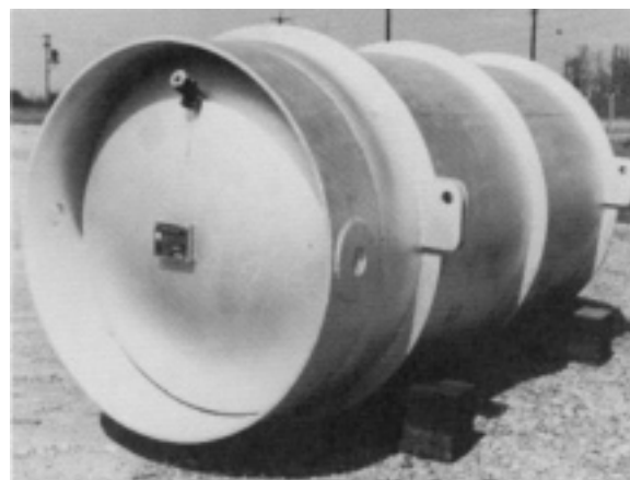
Figure 1.6. Cylinder for transporting uranium hexafluoride.
