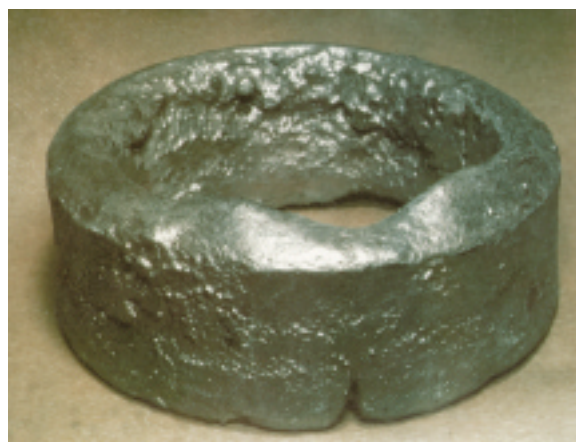
Figure 1.5. Plutonium ring (~14 cm in diameter) produced by electrorefining.
