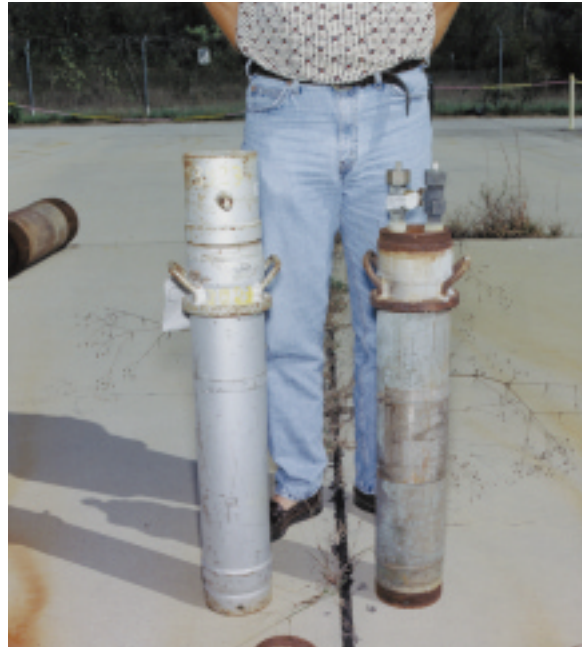
Figure 1.7. Cylinders (12.7 cm diameter, 1 m length) used for transporting highly enriched uranium hexafluoride.
